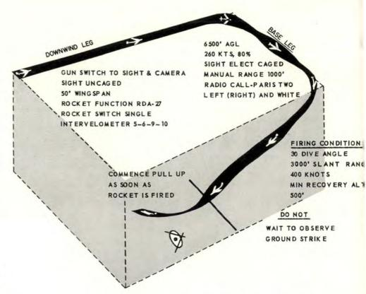
Above is illustration of the typical low-angle rocketry pattern. Fouls lead to disqualification.
