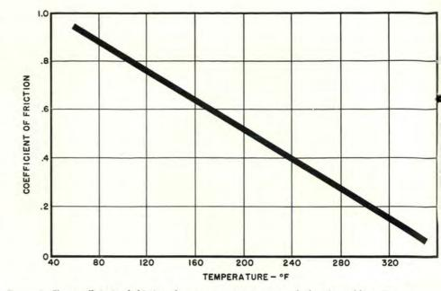
Figure 1. The coefficient of friction decreases as temperature of the tire rubber rises.
