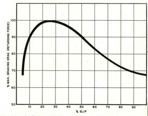
Figure 2. Note the effectiveness of braking versus tire slippage. Some slippage is needed.
