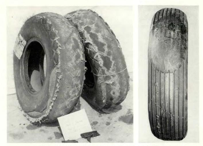
With the installation of anti-skid brakes, getting tires into this condition is almost eliminated.
